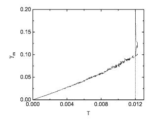
FIG. 7. The Lindemann parameter  $\gamma_m$  vs *T*. The critical temperature  $T_m$ =0.0120 is visualized by the vertical dotted line.
