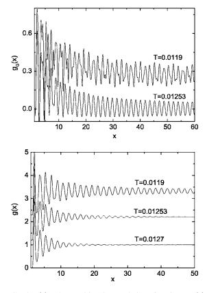
FIG. 4. (a) The positional correlation function  $g_G(x)$  at T=0.01253 in the hexatic phase (lower curve) and 0.0119 in the solid phase (upper curve) plotted vs *x* on a linear scale. (b) The pair distribution function g(x) plotted vs *x* on a linear scale. The upper two curve are shifted upward for clarity. The curves at T=0.0119, T=0.01253, and T=0.0127 show features in the solid, hexatic, and liquid phases.
