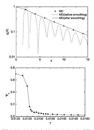
FIG. 1. (a)  $g_6(x)$  obtained with molecular dynamics (MD) and Monte Carlo (MC) simulations at T=0.0150 plotted vs x on a semilog scale. The smoothed curve is shifted upward for clarity. The smoothing technique is described in Section II. (b)  $\Psi_6$  plotted vs T on a linear plot. The bond orientational order parameter increases abruptly around T=0.0125. The line fitted to the circles is a guide to the eyes.
