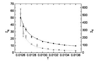
FIG. 2. Bond orientational correlation length (full symbols) and susceptibility (open symbols) as a function of temperature. The curves show the best fits of Eqs. (16) and (17) according to the KTHNY theory. The fitted transition temperatures are  $T_i$ =0.012 37(16) and 0.012 43(4) for the correlation length and susceptibility, respectively.
